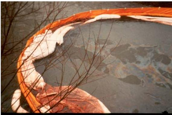
Since the sheen is very thin, it is not practical to use mechanical systems such as skimmers to remove the oil from the water. The most practical method is to use a combination of oil boom and sorbent pads as shown in figure 5. Sorbent pads can be made of either natural materials such as straw or activated peat moss, or synthetic materials like polypropylene. Under field conditions, it is very difficult to
