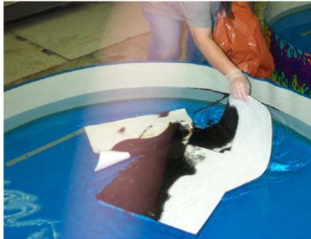
**Figure 6. Sorbent pads used in calm conditions**
