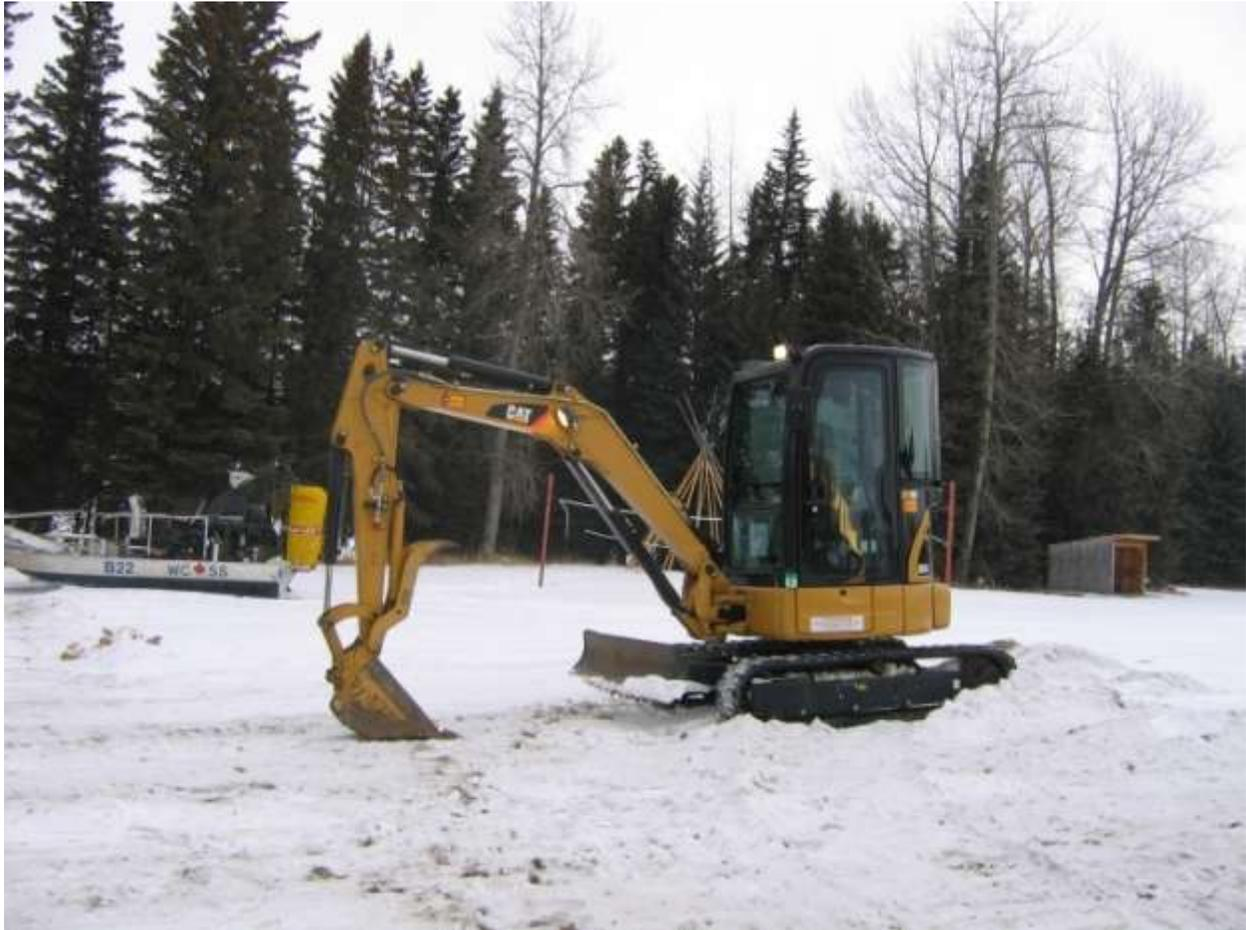
The ice assessment indicated that the ice thickness varied from .4m to .6m. Although the weight bearing capacity graph indicated that it would have been safe to take the equipment onto the ice, the operators were reluctant to do so for an exercise, so the demonstration was conducted with the backhoe's working off the shore on dry ground.
