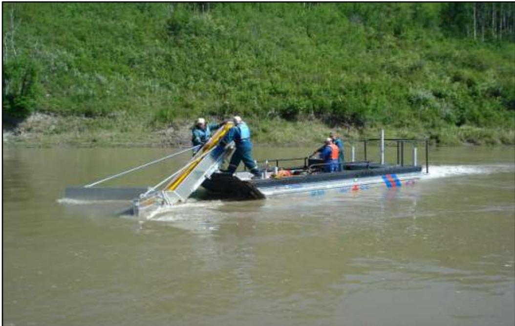
Bow Collector mounted on WCSS barge
